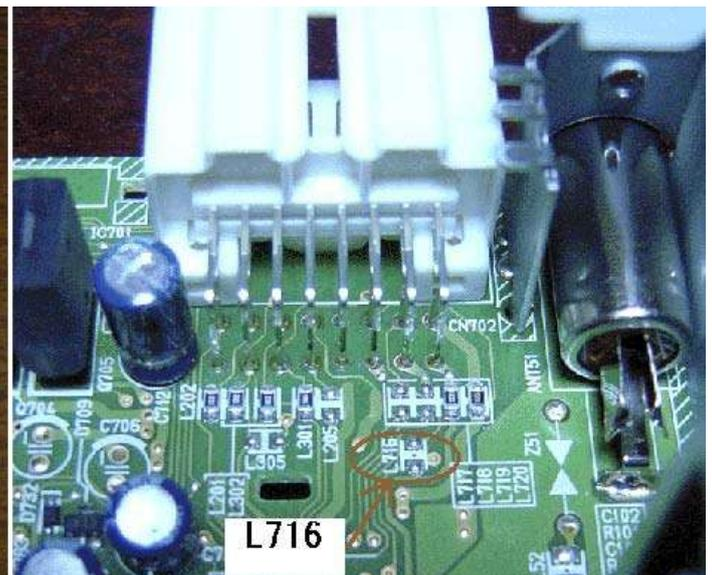
Bridge L716 soldering pads with thin wire and be careful not to short other circuits
