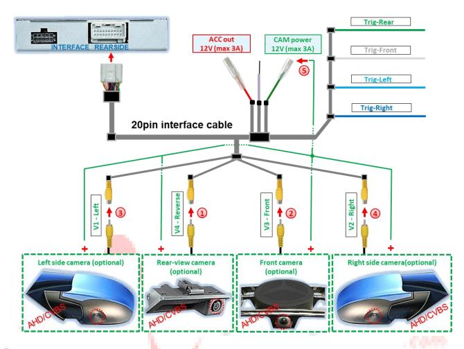
2.5.1 Connection and power-supply - video-sources rear-view camera, front camera and 2 side-cameras
