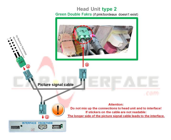
Connect the picture signal cable's waterblue coloured female Double Fakra connector to the male double Fakra connector of the video interface.
