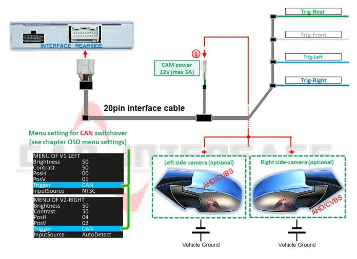
Power supply for side-cameras should be connected to green wire CAM power 12V (max 3A) of 20pin interface cable, as this cable is only powered during camera activation (some cameras are not continuously current stable).
