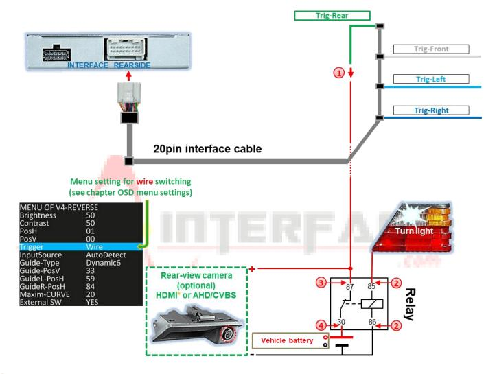
Connect green wire Trig-Rear to output connector (87) of relay.
