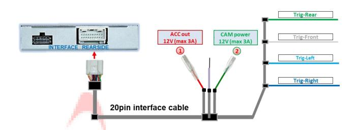
External video-sources (no cameras) can be supplied with power via the red power supply cable ACC out 12V (max 3A) of the 20pin interface cable. The cable carries +12V ACC trigger out power permanently while interface is powered (see following chapters for connection).
