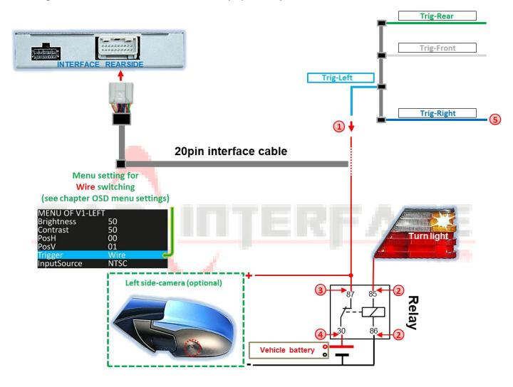
Connect light blue wire Trig-Left to output connector (87) of relay.
