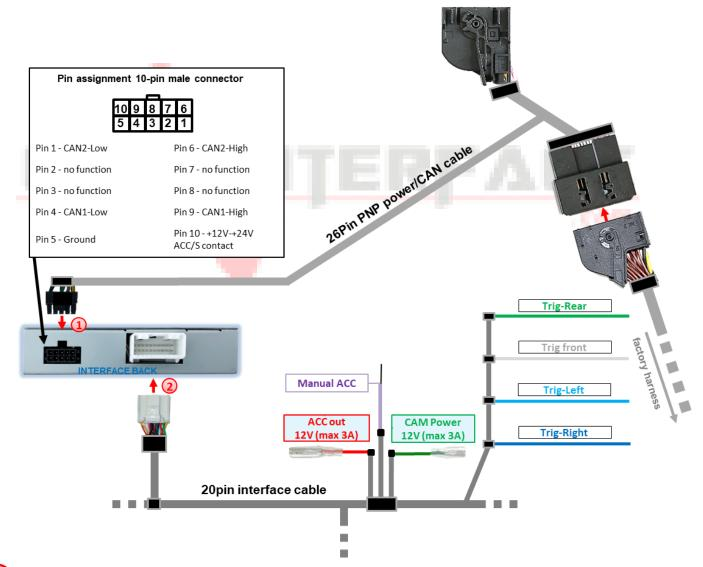
Connect the 10pin female connector of the 26pin PNP power/CAN cable to the 10pin male connector of the interface.
