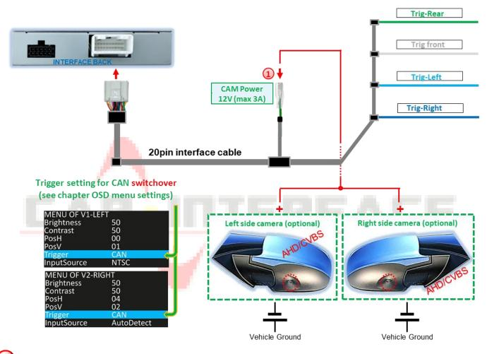
The power supply for the side cameras can be supplied via the green CAM Power 12V wire (max 3A) of the 20pin interface cable, as this wire is only energised during an active video input (some cameras are not suitable for continuous operation).
