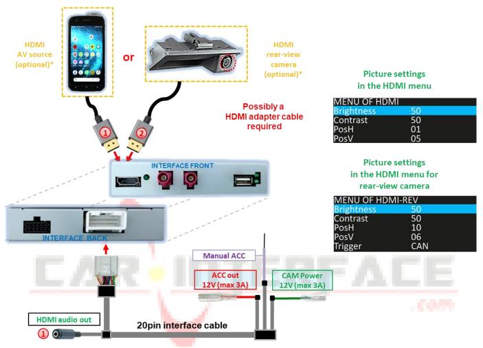
If an optional video source is connected to the HDMI input\*, the picture shown on the display of the source (e.g. smartphone, laptop, etc.) is mirrored on the vehicle monitor. Other sources (e.g. streaming stick, DVD player, DVB-T tuner, etc.) can also be displayed on the vehicle monitor. The video source can be supplied with power via the red wire ACC out 12V(max3A).
