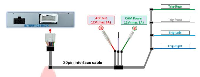
External video sources (no cameras) can be supplied with power via the red ACC out 12V (max 3A) power supply line of the 20pin interface cable.
