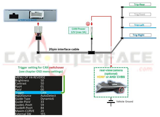
The +12V power supply for the after-market rear-view camera can be provided via the green wire CAM Power 12V (max 3A) of the 20pin interface cable, as voltage is only present on this wire when one of the video inputs is active (some cameras are not suitable for continuous operation).
