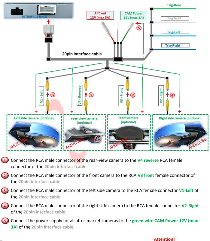
2.5.1 Connection and power supply - Video sources Rear-view camera, front camera and 2 side cameras
