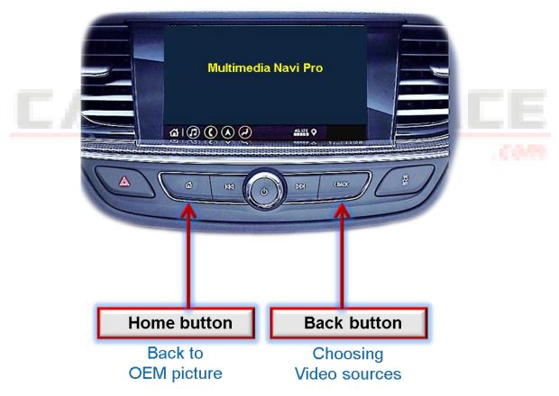
Switchover by vehicle buttons isn't possible in all vehicles. In some vehicles the external keypad has to be used.
