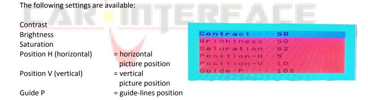
**Note:** If there is no communication between interface and the vehicle's CAN-bus (several vehicles aren't compatible), the optical PDC and the reverse gear guide-lines can't be shown during the vehicle's operation, even if they once appear after having switched the system to powerless!
