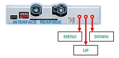
The picture settings are adjustable by the 3 push-buttons at the rear-side of the video-interface. Press the MENU button to open the OSD settings menu or to switch to the next menu item. Press UP and DOWN to change the selected value. The buttons are placed inside in the housing to avoid accidental changes during or after the installation. Picture settings must be done separately for all video inpouts while the corresponding input is selected and visible on the monitor.
