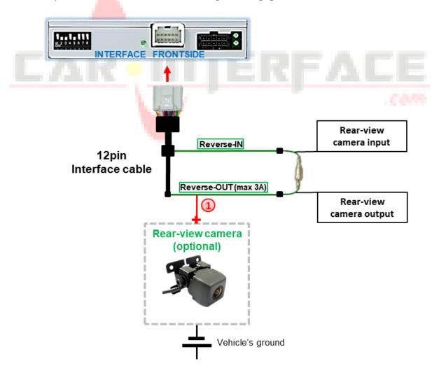
Additionally, the +12V (max. 3A) power supply for the rear-view camera can be taken from the green wire of the 12pin interface cable.
