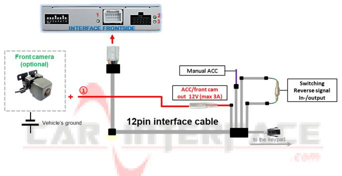
1 The red power supply output ACC/front cam out 12V (max 3A) can be used to power a front camera. If Dip 1 is set to ON (black 8 dips), the power supply output gives +12V (max 3A) when reverse gear is engaged plus 10 seconds delay after reverse gear is disengaged.
