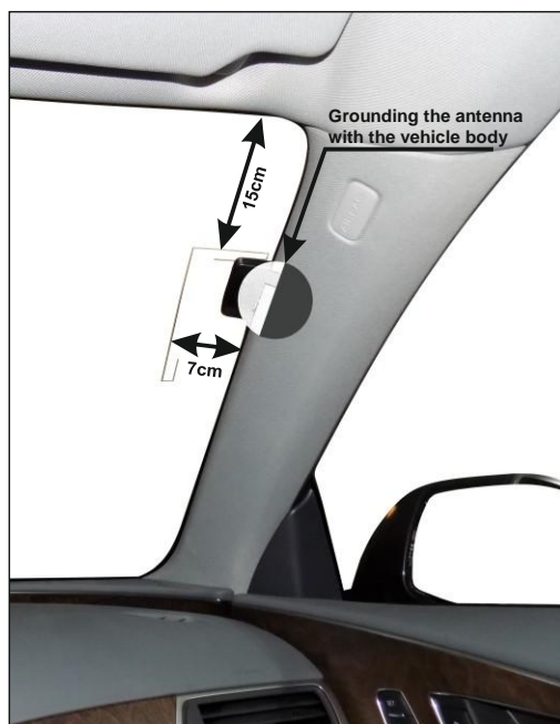
Example of mounting a DAB/DAB+ antenna
